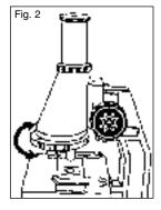
CAUTION: Be careful as you turn the focus knob so that the objective lens does not make contact with a slide or the stage. This may cause damage to the slide and also to the objective lens.
